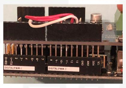
Place the pins in the socket and gently and with even pressure connect the two sections together.
